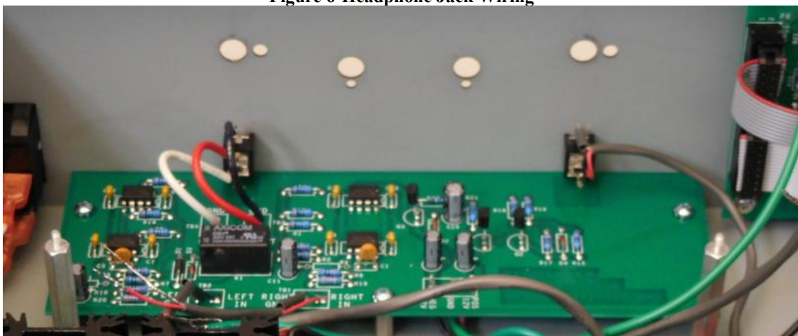
Figure 7-Headphone Amp Installed with jack wiring completed
