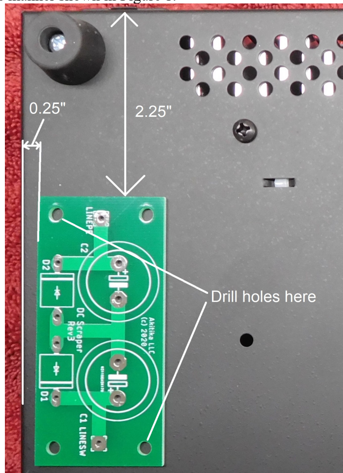
Figure 1-Using the PCB to locate the 2 new mounting holes
