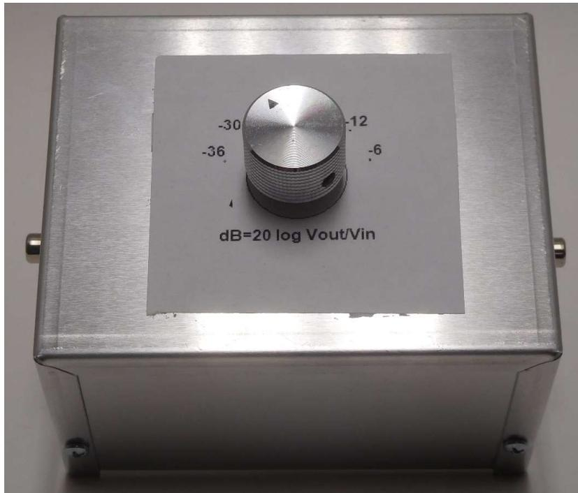
Figure 1 – Assembled attenuator, built by Dan
