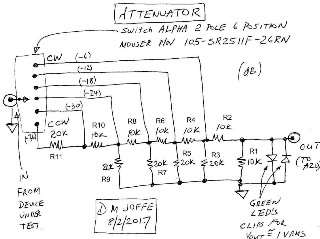
The amplifier under test connects to the RCA jack on the left side of the schematic. From there, the signal connects to a 6-position selector switch. The attenuation of the switch increases as the selector turns counter-clockwise.
