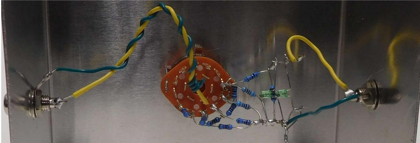
Figure 2 – Inside the assembled attenuator. Green wire from the input (left) RCA is twisted and wrapped around the yellow wire to form a shield. It is not connected anywhere on the switch.
