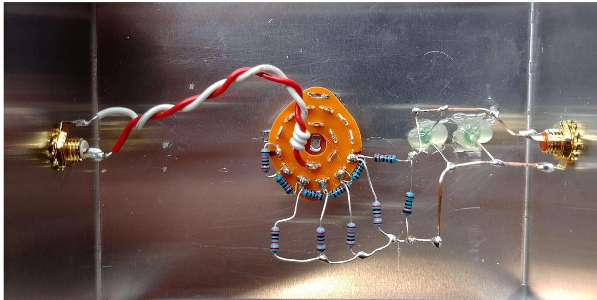
Figure 3 – Craig's layout is neater than mine. Note that he made the LED's visible, so you can see when you're over-driving the A2D, and hence are in protection mode.
