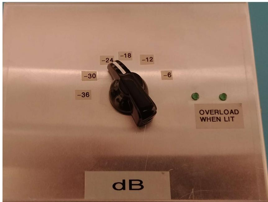
Figure 2 – assembled version, as built by Craig, with LED's visible to show overload
