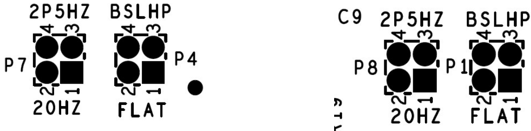
Figure 10-Left Channel and Right Channel High Pass Jumpers
