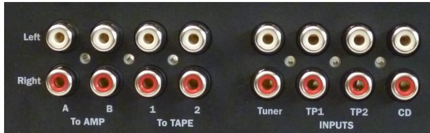
Figure 44-Install plastite screws (6) in the holes between the left and right channel input jacks
