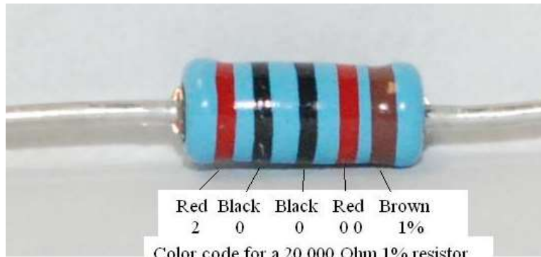
Figure 46-demonstrating the resistor color code
