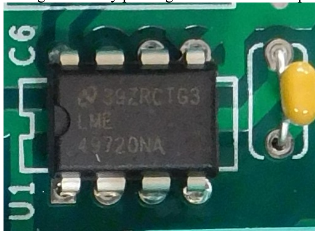
Figure 3-Detail shows correct orientation for U1
