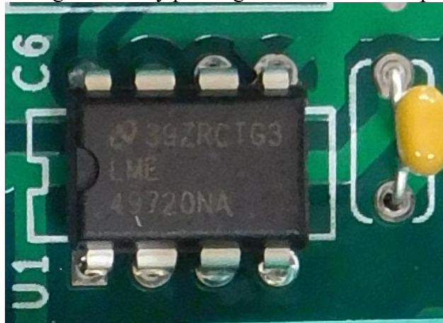
Figure 3-Detail shows correct orientation for U1
