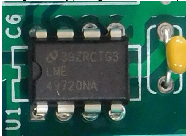
Figure 3-Detail shows correct orientation for U1
