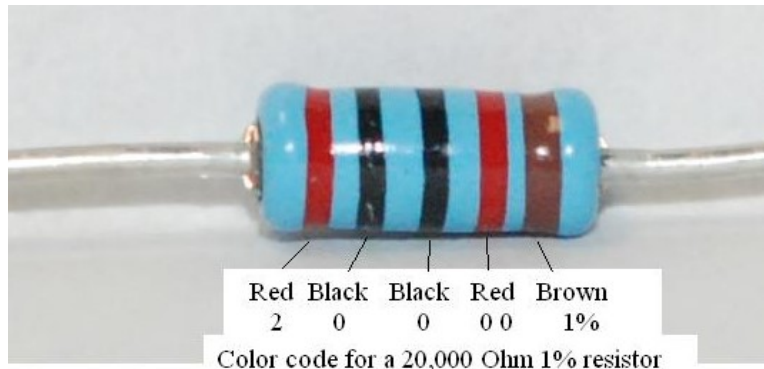
Figure 7-demonstrating the resistor color code
