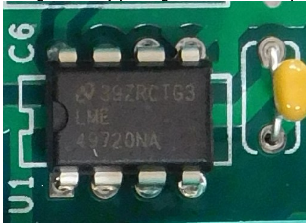
Figure 3-Detail shows correct orientation for U1
