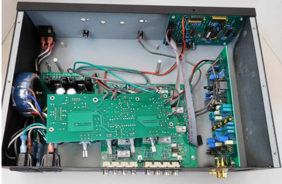
Figure 5-Tone/Volume dismantled to make room to install Headphone Amp
