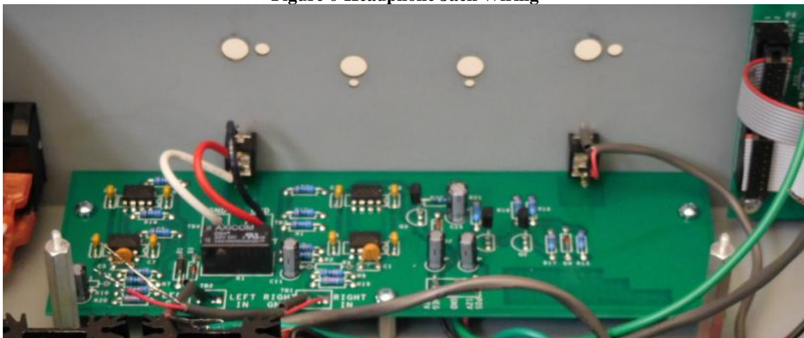
Figure 7-Headphone Amp Installed with jack wiring completed
