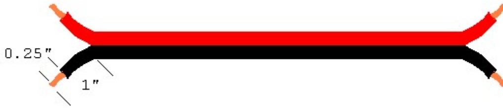
Figure 4-Prepare 12" length of Red/Black Zip cord (drawing not to scale)
