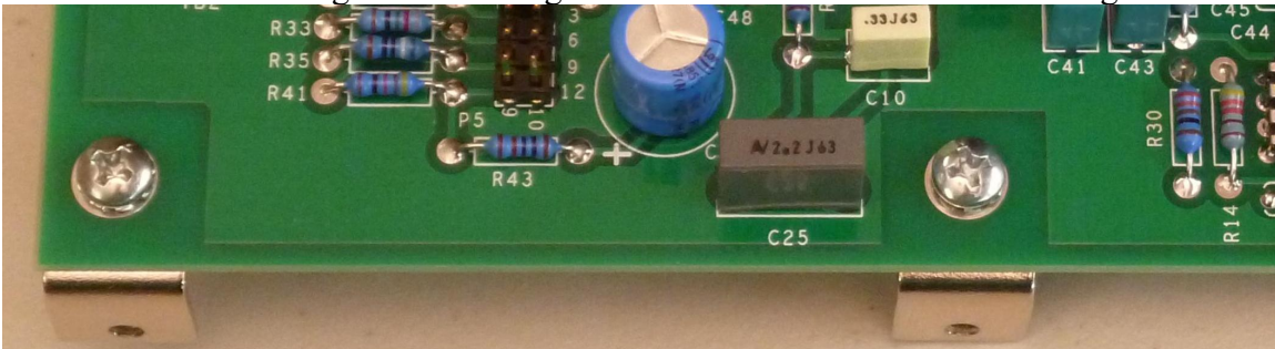
Figure 8-Install the mounting brackets
