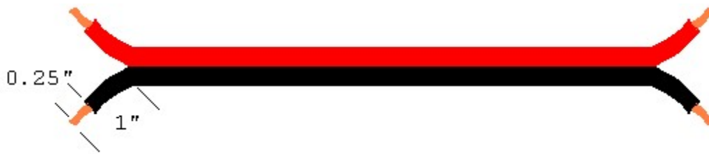
Figure 4-Prepare 12" length of Red/Black Zip cord (drawing not to scale)
