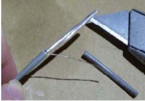
5. Separate and twist the drain wire.
