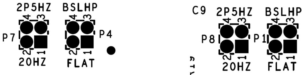
Figure 10-Left Channel and Right Channel High Pass Jumpers
