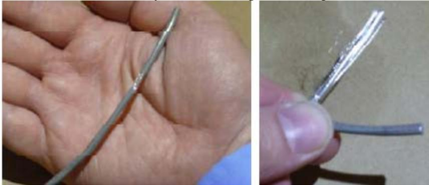
3. If you've scored the jacket carefully, you can separate the jacket at the score line without using tools. Pull the insulating jacket off, exposing the cable, showing the foil shield, the drain wire, and the fuzzy string. The result is shown here, with the foil shield showing.
