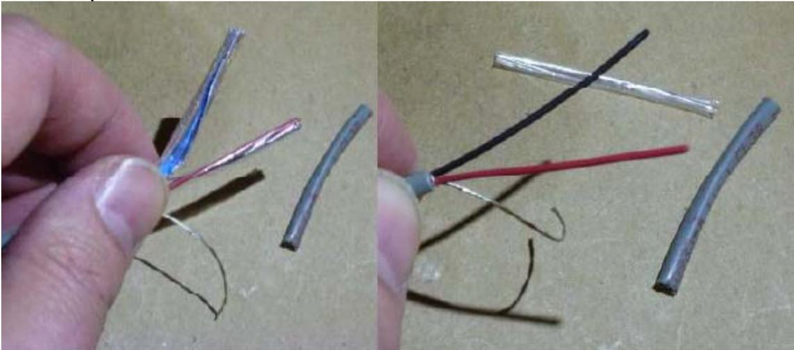
6. Peel back and remove the foil. Remove the plastic wrap from the red and black wires. The drain (bare wire), red, and black wires are exposed now that gray insulating jacket, foil shield, and plastic over-wrap have been removed.
