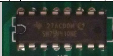
Figure 36-Remember to match silk screen and IC orientation mark
