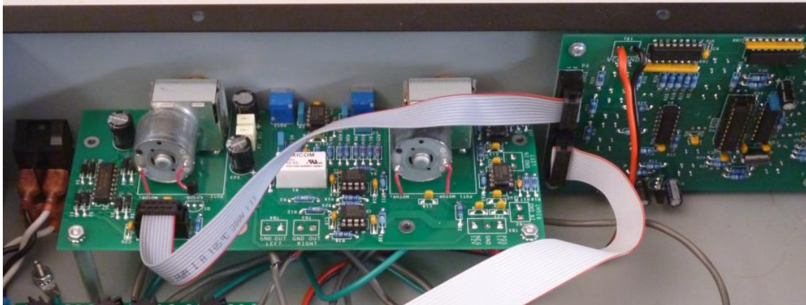
Figure 43-Showing 10 pin Ribbon Cable Installation and Orientation
