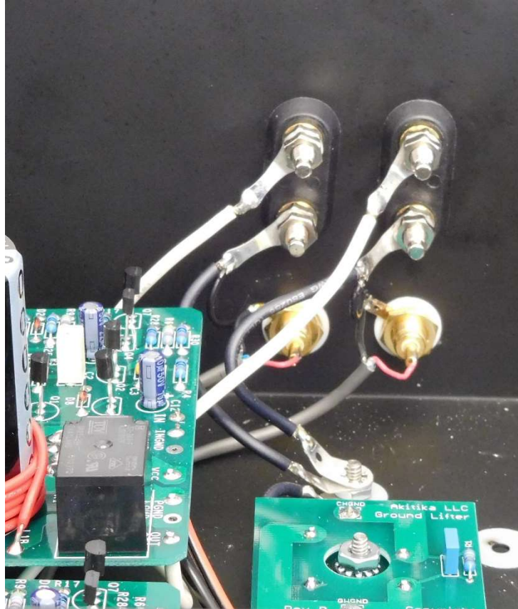
Figure 38-I/O Connector wiring
