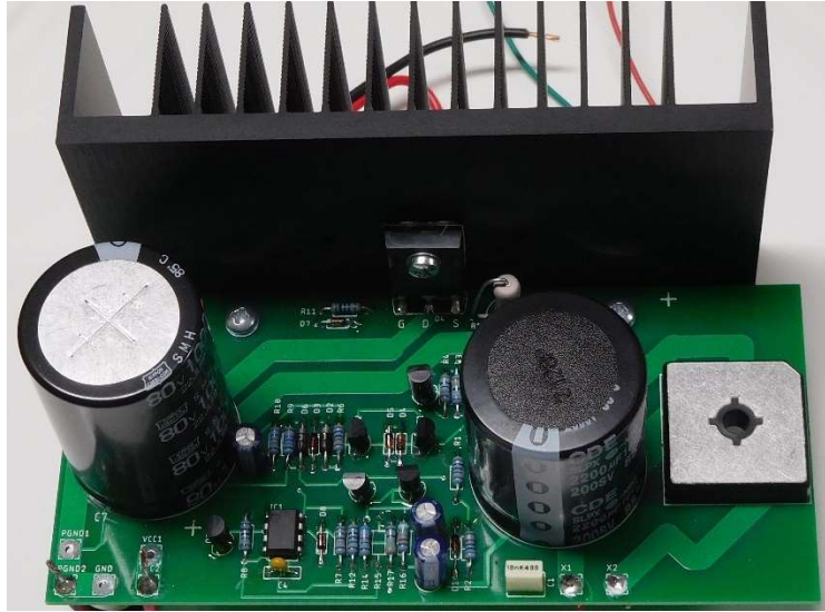
Figure 6-Installing Q4 on the heatsink and to the PCB
