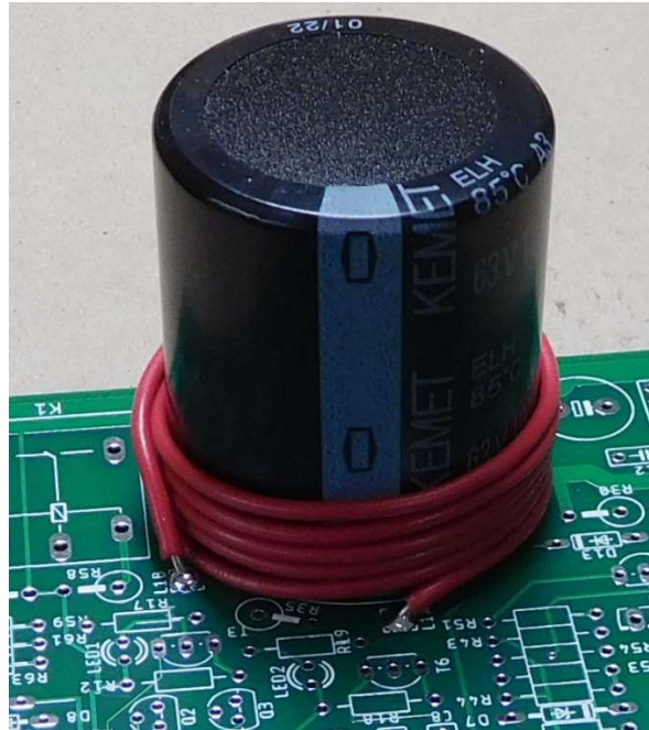
Figure 13-Winding the output inductor
