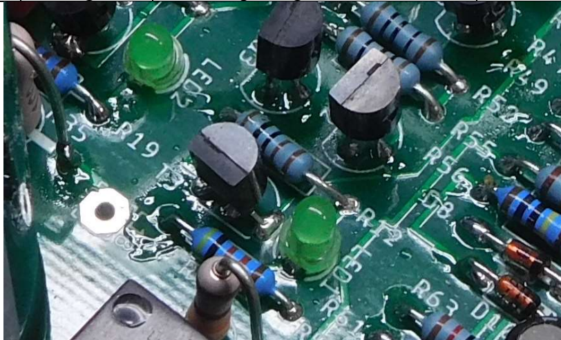
Figure 10-Note flat side of LED package sits under number 1 and 2 in LED1 and LED2
