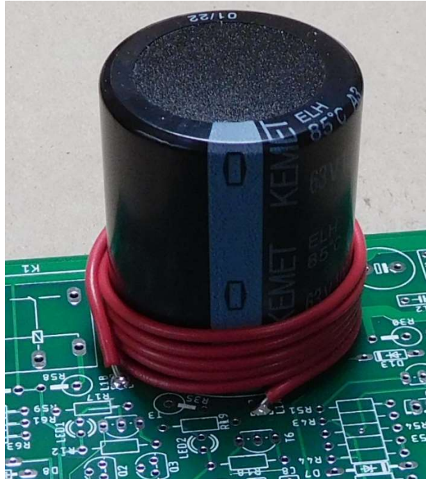
Figure 13-Winding the output inductor
