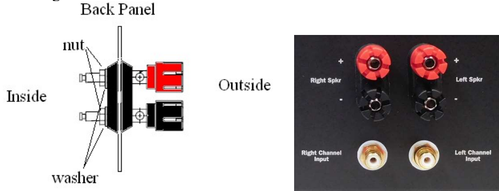
Figure 37-Install both left and right binding posts
