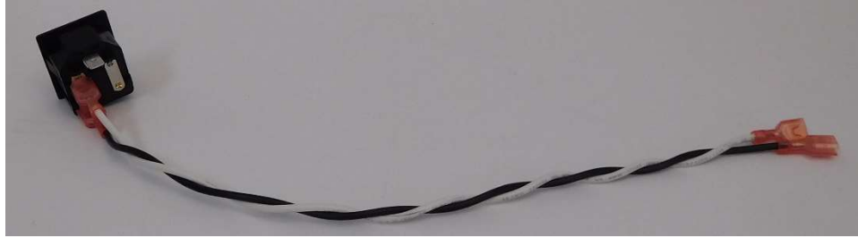
Figure 33-Wiring IEC power connector line and neutral
