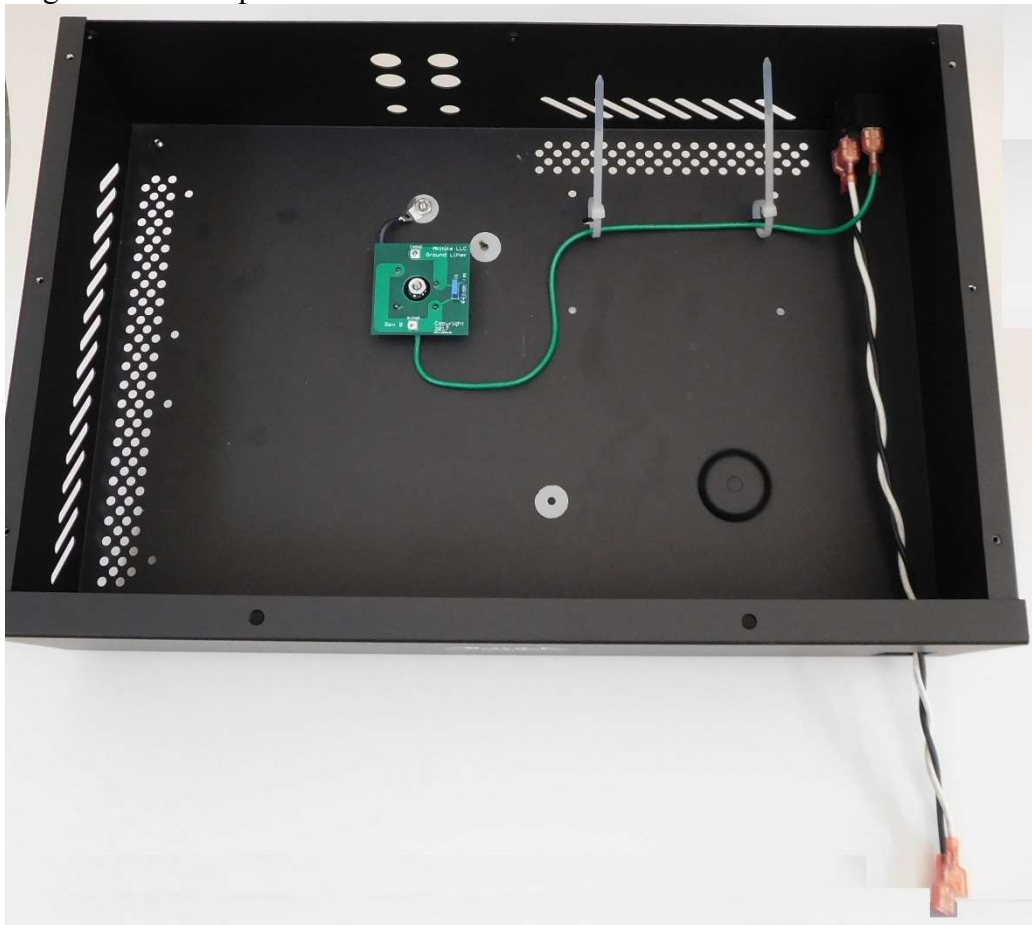
Figure 38-Power wiring with IEC connector installed into chassis
